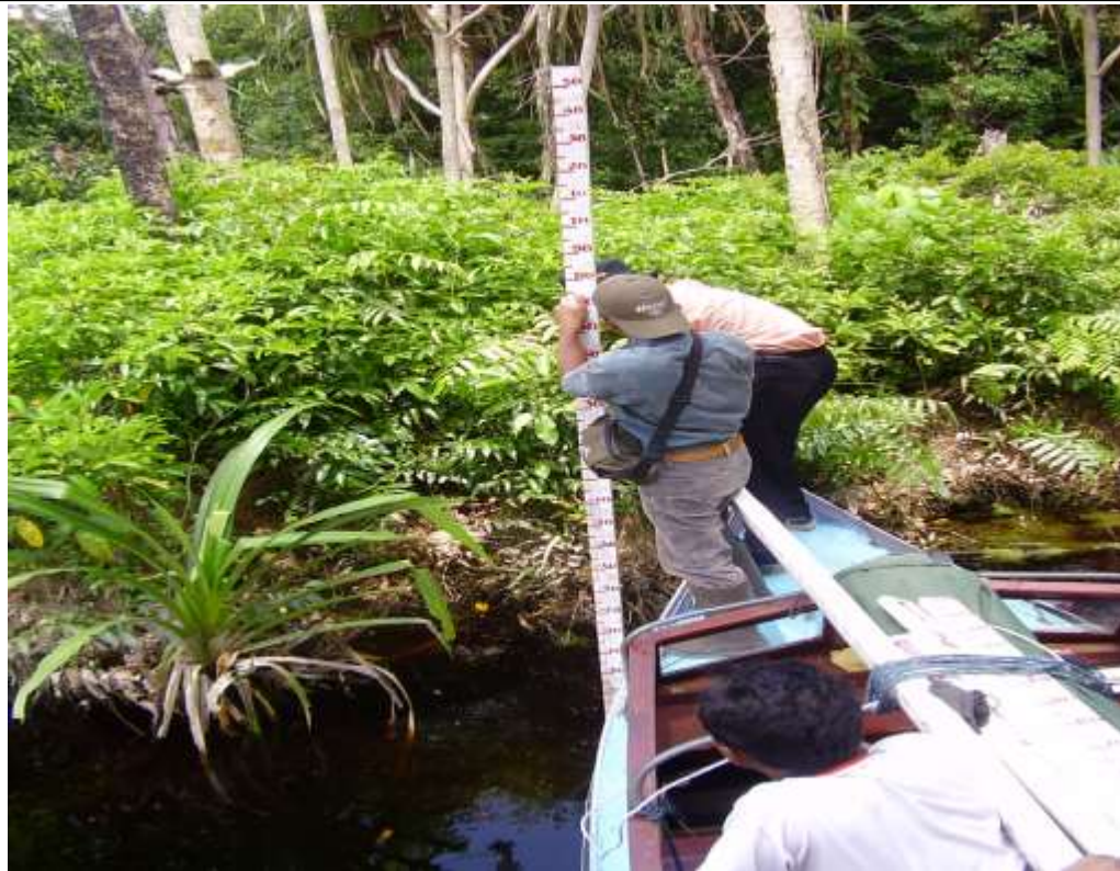
Installation of water-level gauge to measure fluctuation in water level.
