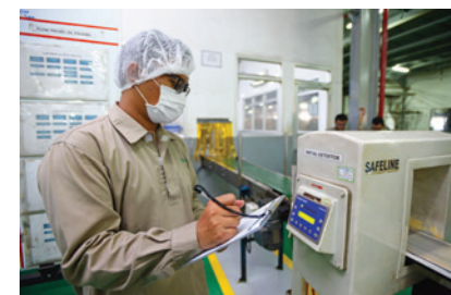
Strict quality control processes such as screening of products through a metal elements detector
